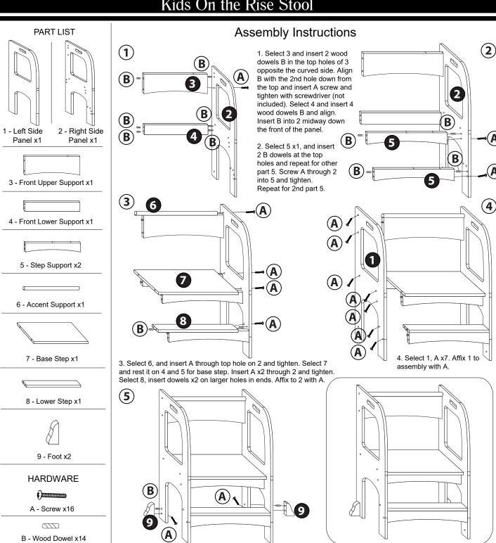
5. Select 9 x1, insert B into larger hole of 9. Insert B
